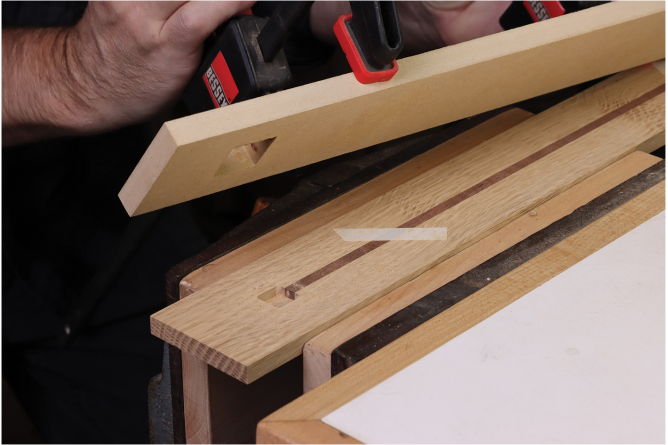
12 A pair of clamps help break the template free. Note how the router has now defined the length of the walnut strip automatically.
