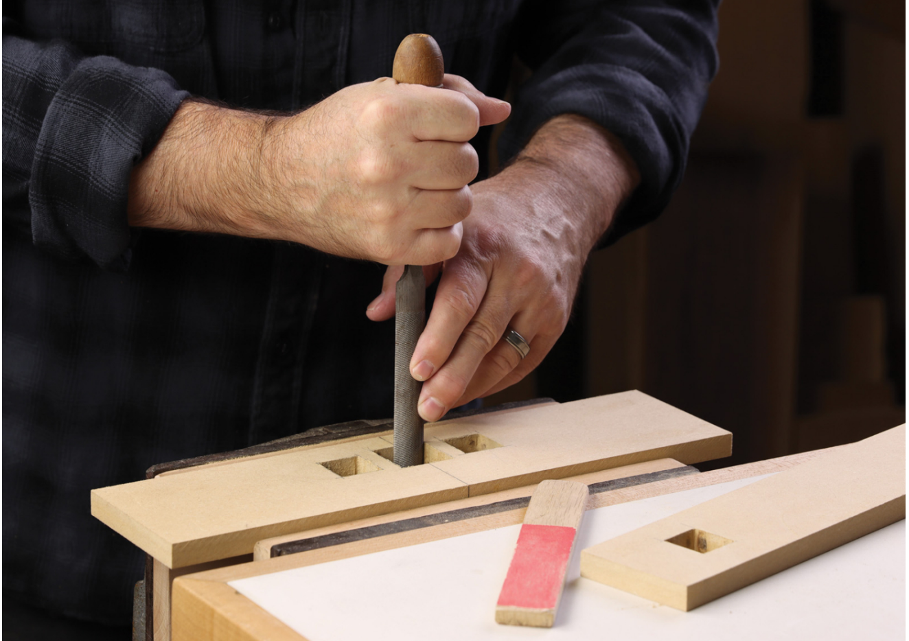
4 Cut out the openings and use a file or sanding block to fine-tune the 1/2" MDF inlay templates.
