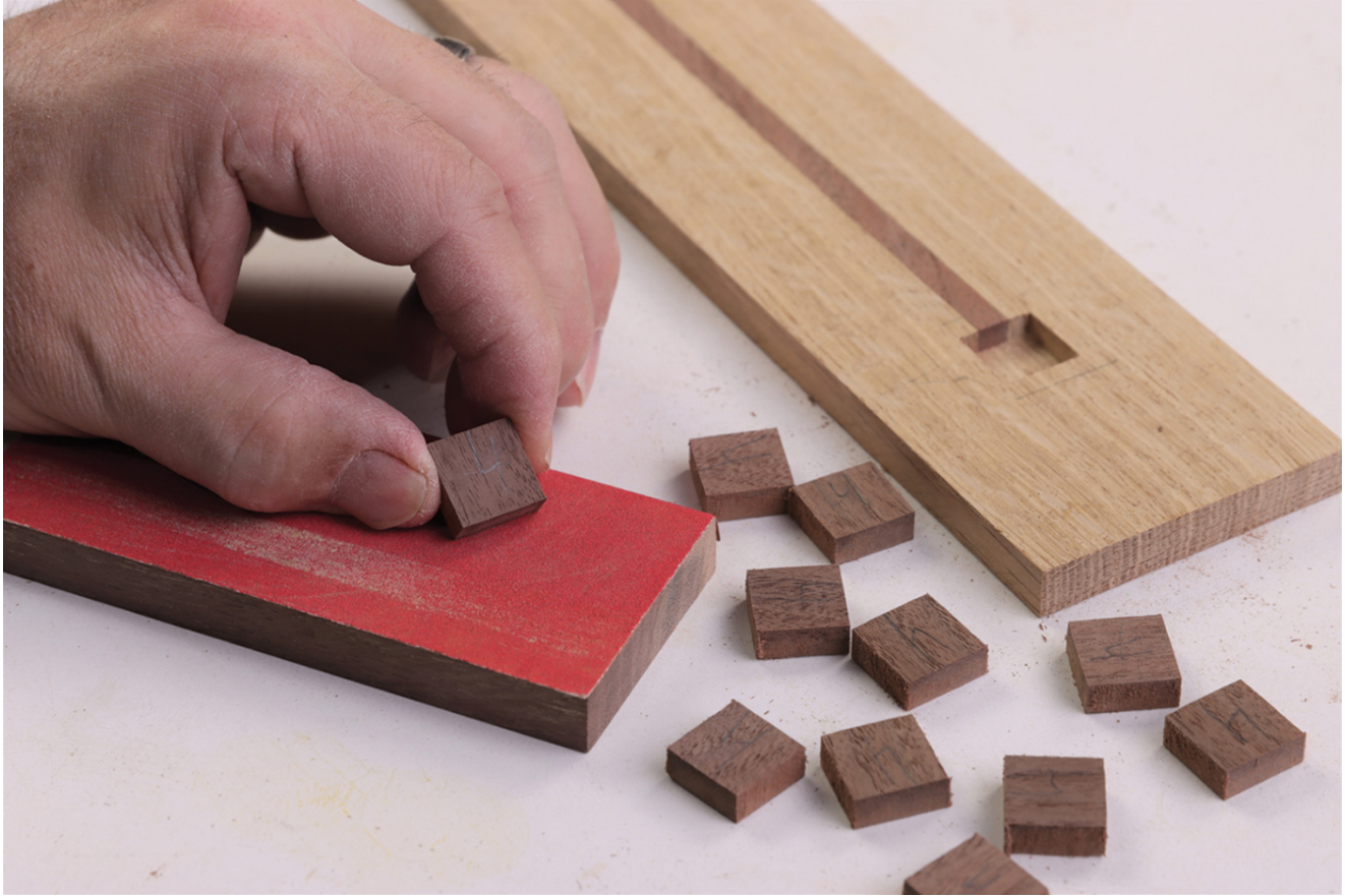
15 Painter's tape holds the squares in place and prevents damage as you make the cut.
