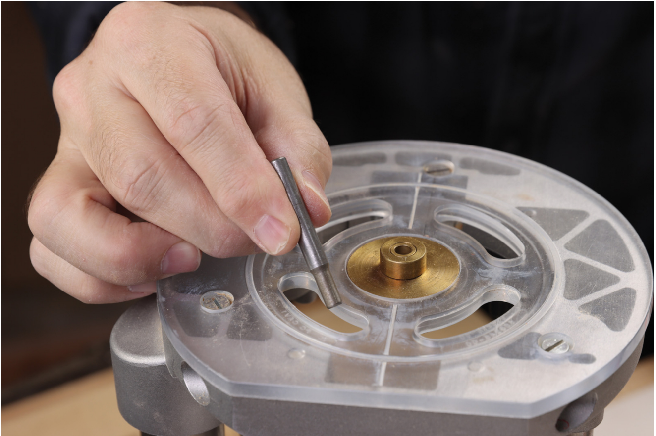
6 Prepare your plunge router by installing an inlay bushing kit. Some kits, such as Whiteside #9500, come with a special centering rod to center your router sub-base.
