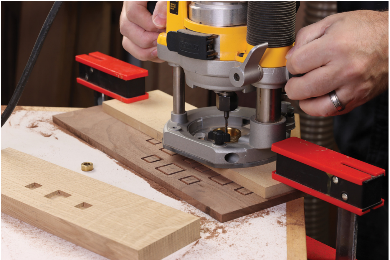
12 A pair of clamps help break the template free. Note how the router has now defined the length of the walnut strip automatically.
