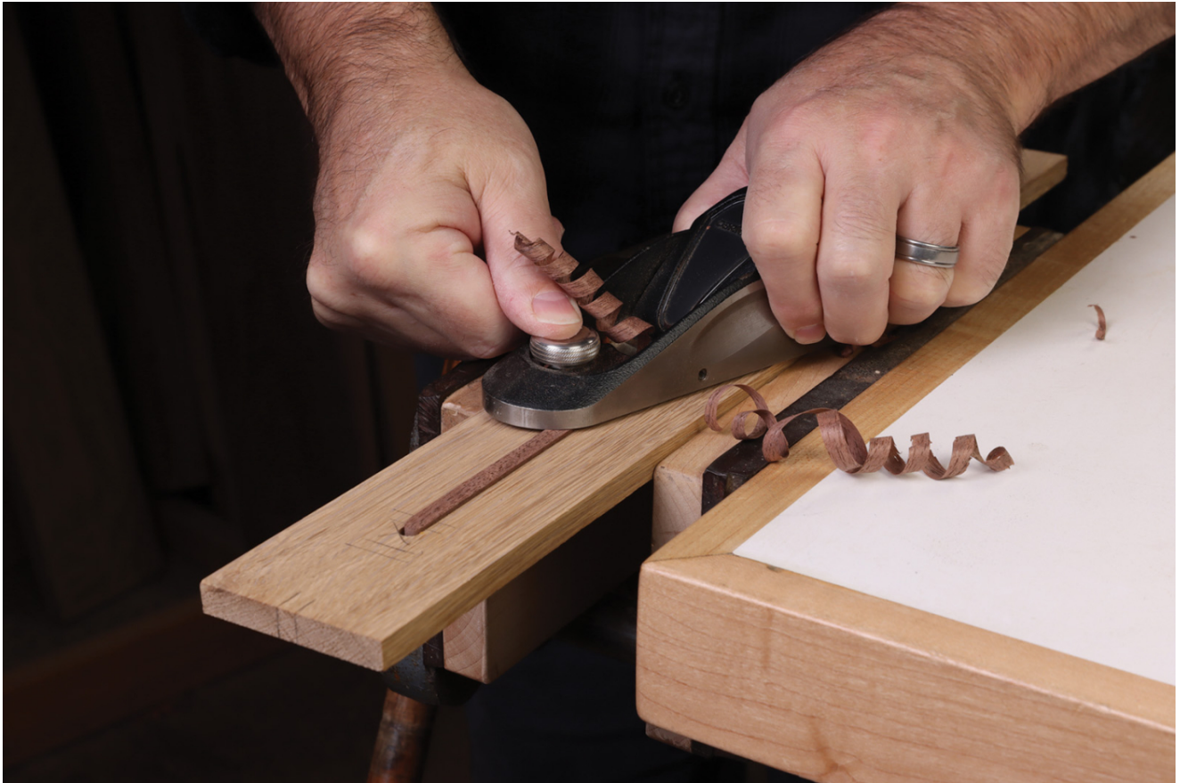
9 Rout a centered groove in the slats and glue in a 1/4" wide strip of walnut.
