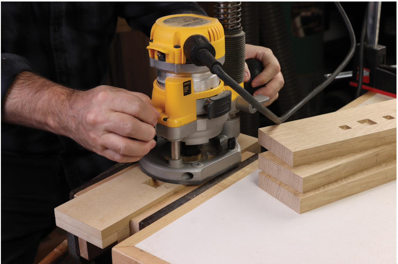
6 Prepare your plunge router by installing an inlay bushing kit. Some kits, such as Whiteside #9500, come with a special centering rod to center your router sub-base.
