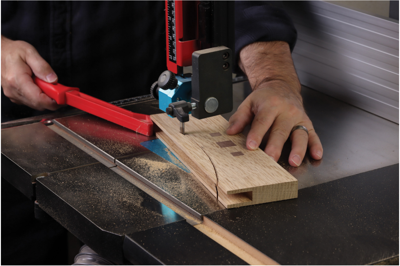
19 Band saw the curve just outside your layout line.
